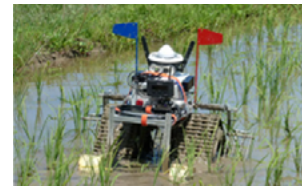
[ Robot equipped with AI-supported image recognition for weeding rice paddies ]
