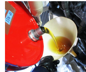
[ Replacing lubricating oil ]
