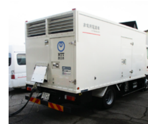
[ NTT West's emergency power supply vehicle ]
